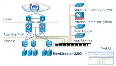
The FlowDirector can help network administrators to manage monitoring network without service interruption. Also it helps network administrator load balance the traffic across multiple monitoring devices to provide the analytical processing power to where it is critically needed.
